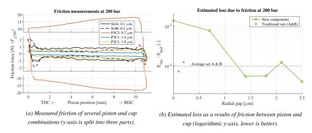
Figure 8: Friction measurements of several piston and cup combinations at 200 bar (Shell Tellus46 at 50°C).
