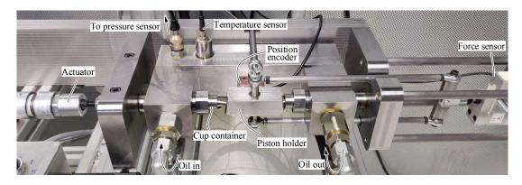
Figure 6: Picture of the actual testbench.
