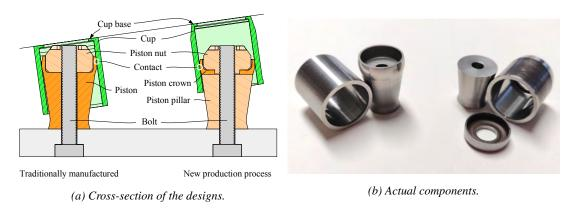
Figure 1: Comparison between the traditionally manufactured components and the new components.
