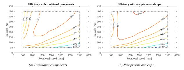
Figure 12: Efficiency field of the prototype 45 cc floating cup pump with traditionally manufactured components (a) and pistons and cup that were made using the new production process (b).
