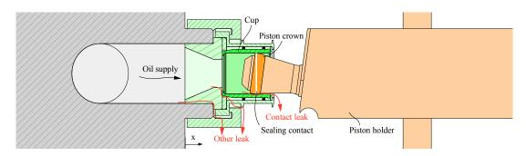
Figure 7: Cross section of the cup container, showing the cup, the piston, and the sealing contact between these two components. The red arrows show three leak paths.
