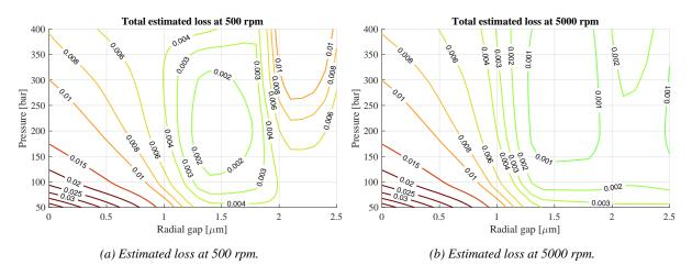
Figure 10: Estimated total loss as a function of gap size and pressure levels (lower is better).
