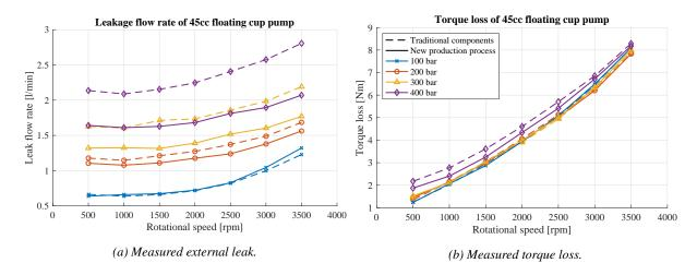
Figure 11: Performance measurements of the prototype 45 cc floating cup pump with traditionally manufactured components (dashed lines) and pistons and cup that were made using the new production process (solid lines).
