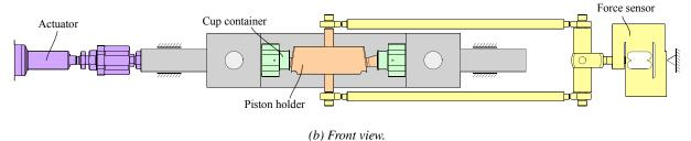
Figure 5: Sketch of the testbench for testing individual pistons and cups viewed from top (a) and front (b). The actuator (purple) moves the steel frame (gray) including the cup containers (green) and position encoder (blue) in the direction of x, while the piston holder (orange) is kept stationary by the force sensor (yellow).
