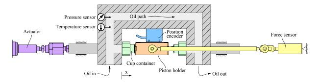
(a) Top view, with cross-section of the steel frame, showing the path of the oil.
