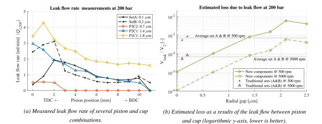
Figure 9: Leak measurements of several piston and cup combinations at 200 bar (Shell Tellus46 at 50°C).
