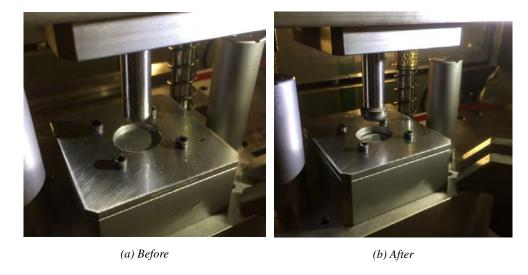
Figure 2: First phase (deep drawing) of the production process of the cup on a prototyping press.
